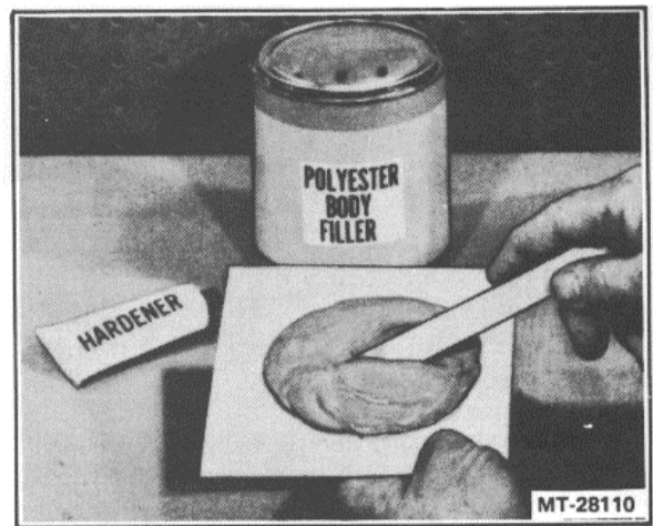
Figure 11. - Preparing Body Filler
