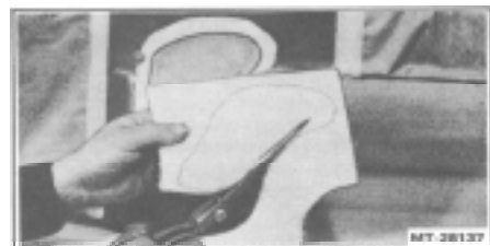
Figure 39. - Cutting Mat For Filler
