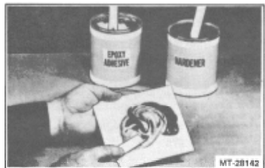
Figure 44. - Mixing Epoxy Adhesive
